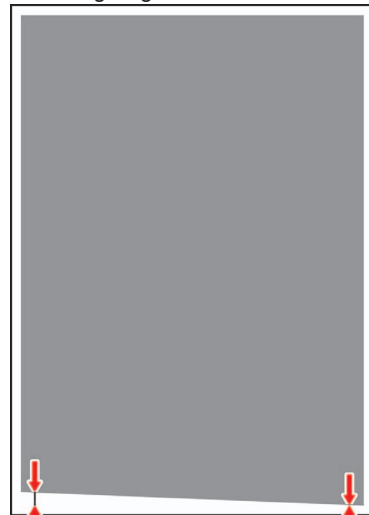
6. Poor Parallel Reproduction Along Trailing Edge
